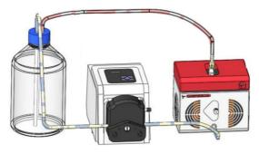
Reservoir → reservoir outlet → chamber inlet → ETC Chamber → chamber outlet → reservoir inlet → Reservoir
