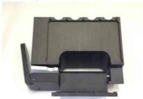
Use this device in order to easily open tray's frame. Push first the holder in front of it and then the one on the left side. Place your slides face up with the label in between the holder, then press the silver button to open the device.
