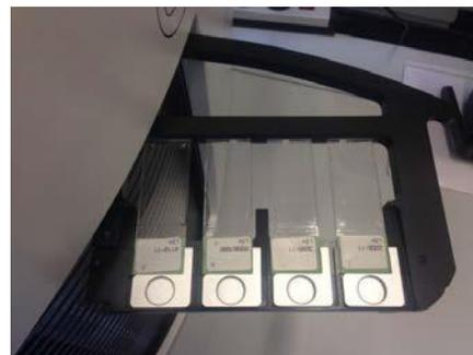
"Open" the slide scanner in order to insert trays. Please take extra care when you select a free slot. A slot is free when there is no light (grey).
